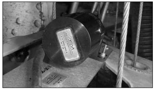
SpaceAge Control position transducer shown mounted near 727 flight control cable as part of ASM FDR upgrade kit. Photo courtesy of Aircraft Systems & Manufacturing Inc.
