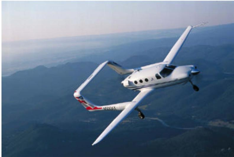
The A500 on its first flight with SpaceAge Control air data and displacement measurement sensors aboard.
