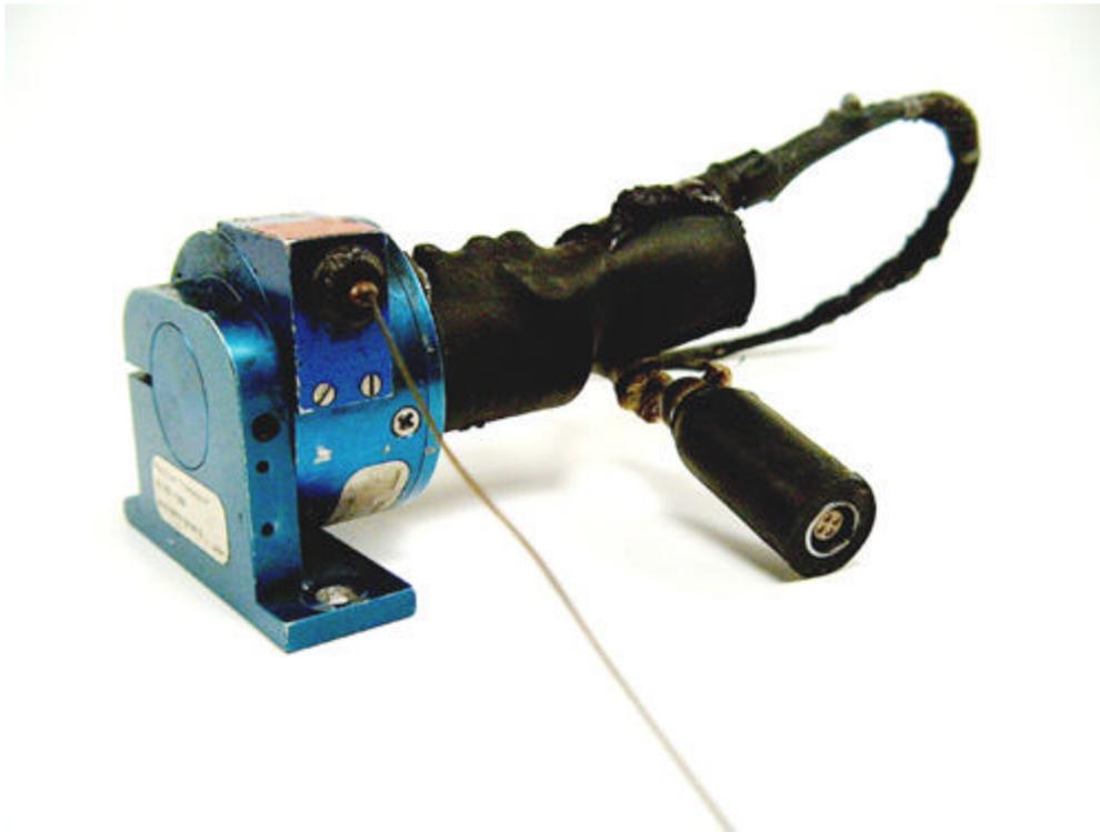
It survived: The Series 160 sensor was battered and burned but passed all acceptance testing after the crash.
