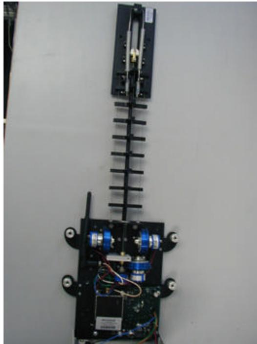
Frame of device showing 3 displacement sensors mounted.
