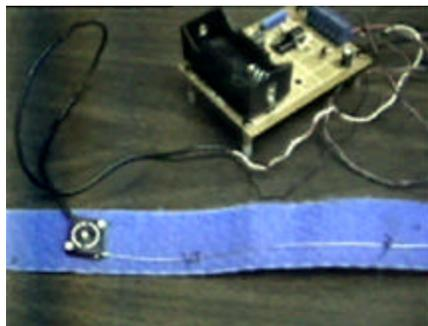
Series 150 position transducer shown on mounted on organ motion belt.
