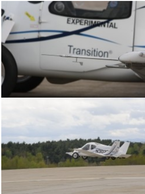
The 100400 air data probe on the left wing-tip of the Terrafugia Transition. ( high-resolution graphic ). The Terrafugia Transition in flight with the 100400 air data probe. ( high-resolution graphic ).
