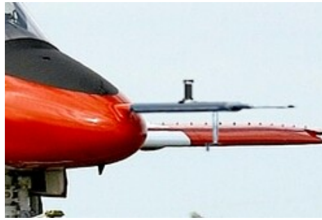
Nose-mounted 100700-051 air data boom (ground)
